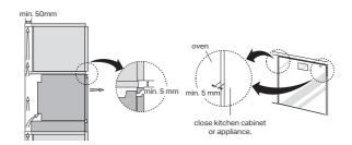
For correct ventilation, the ventilation opening of 5 mm (1.97") should be required between the back wall and the floor of the installation cabinet, the ventilation gap of 5 mm (1.97") is required between the oven top rim and the furniture lower rim, and between the oven both sides rim and the cabinet. These openings must not be closed in any way. So ensure that the sides are not touching the front edges of the housing. Connect the oven to the power supply.
