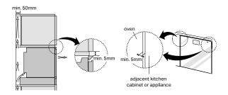
For correct ventilation, the ventilation opening of 50 mm (1.97") should be required between the back wall and the floor of the installation cabinet, the ventilation gap of 5 mm (1.97") is required between the oven top rim and the furniture lower rim, and between the oven both sides rim and the cabinet. These openings must not be closed in any way. Therefore ensure that the sides are not touching the front edges of the housing.
