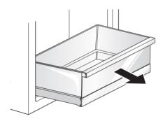
2 Lift the empty drawer slightly to remove it from the support.
