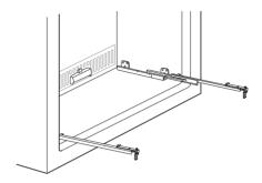
2 Line up the bottom edges on the sides of the drawer support with the groove in each rail and then lower the support until it clicks into place.
