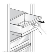
2 Lift the empty drawer slightly to remove it from the support.
