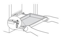
2 Keeping both levers pressed, lift the drawer support slightly and remove it from the rail system.
