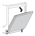
2 Use the door adjustment screws (Φ 4 x 34 mm) provided to adjust the door spring tension at the bottom of the dishwasher.
