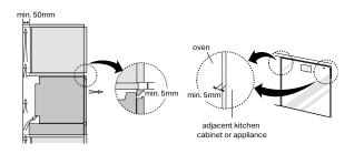
For correct ventilation, the ventilation opening of 50 mm (1.97") should be required between the back wall and the floor of the installation cabinet, the ventilation gap of 5 mm (1.97") is required between the oven top rim and the furniture lower rim, and between the oven both sides rim and the cabinet. These openings must not be closed in any way. Therefore ensure that the sides are not touching the front edges of the housing.
