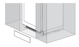
1 Use a screw 1 to attach the bottom cover to the appliance.
