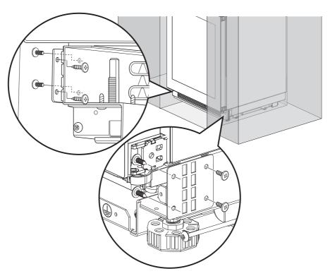
• If there is not enough space to tighten the screw on the side by the baseboard, attach the bracket to the bottom of the adjoining cabinet.
